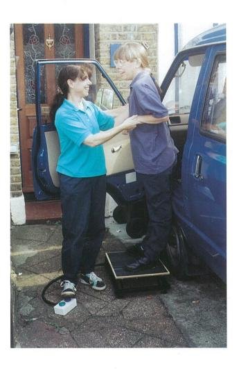
The lift has a wooden platform mounted on a rigid steel frame. A powerful electric motor raises and lowers the platform via a scissor jack mechanism. It is powered through the cigarette lighter socket and operated using a remote foot control button.
