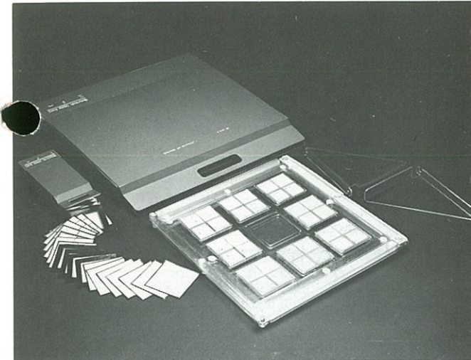
Communication aid for non verbal children, using 'eye-pointing' techniques
